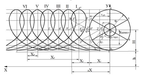
Fig. 1. Interaction of combs of combing drum with plant stems
