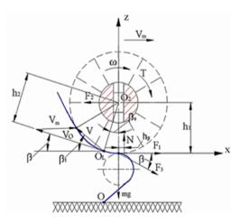
Fig. 2. Forces acting on the brush drum with its free movement in the vertical direction
